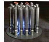
A scale representation of the HIFAR reactor core, showing the cylindrical fuel elements each of about 1m length
