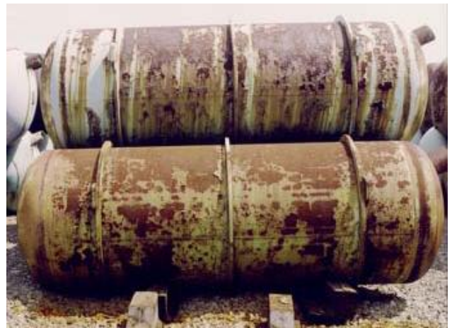
Corroded M48 Containers at Portsmouth
