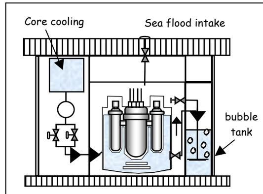
2 Integrated PWR plant (1 of 2) in Compartment No 6 showing schematic of emergency cooling systems
