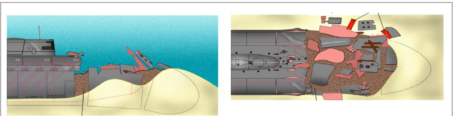
1 The bow damage showing failure of both flood and pressure hulls- internally the damage extended into the boat, collapsing lateral bulkheads into through to N° 5 Compartment - the red cylinders are gas bottles
