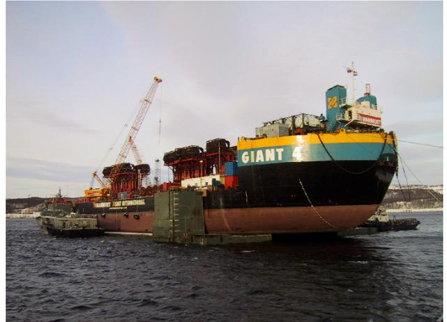
5 Giant 4 with the *Kursk* slung underneath awaits entry into the floating dock at Rosljakovo – two sinkable pontoons were deployed to raise Giant 4 for the necessary clearance into the floating dock
