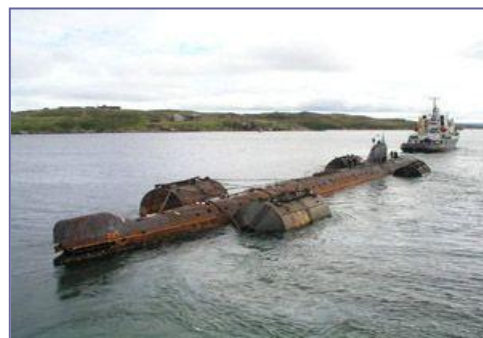
2 K-159 under tow with floatation pontoons
