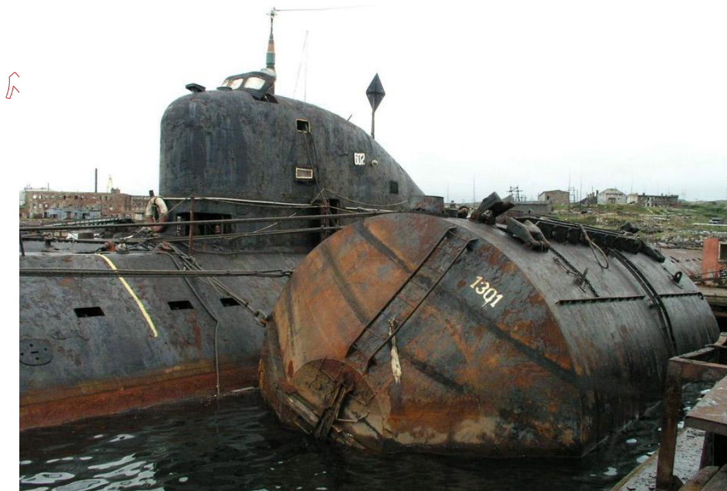
4 Detail of a Floatation Tank and its Hawser Attachment
