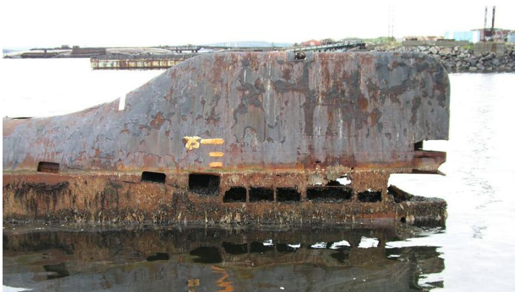
8 Corroded condition of the stern casing
