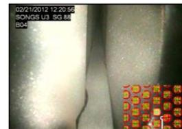
Example of AVB Wear to L/H tube-to-bar
