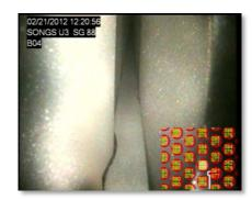
creates a wear scar that is up to x3 deeper than a scar produced by an untwisted AVB {footnote 24} and see  $[p76, Figure 2-18]^{14}$  and other examples where the AV bar has sharply cut into the tube.
