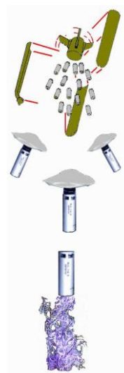
One of 200 canisters of a BLU-114/B submunition which deploys coated carbon fibre strands to short-out and burn through overhead power lines
