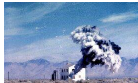
Vapour formation Stage of an FAE
