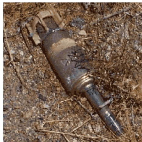
An unexploded but fused Rockeye bomblet showing the inertia impact spike and the twist lock (top) which is rotated by the stabilising fin (out of frame – top)
