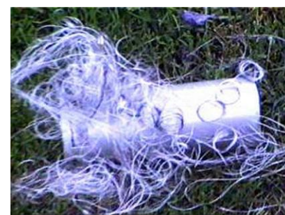
One of 200 canisters of a BLU-114/B submunition which deploys coated carbon fibre strands to short-out and burn through overhead power lines
